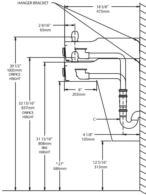
NOTE: A service supply stop must be installed at the cooler inlet tube.
